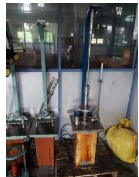
Rammer and Compaction Pedestal
