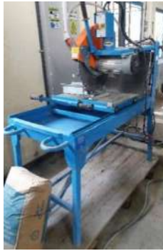
Concrete Cutting Machine
